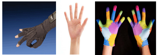
Figure 1. Data glove based, vision based and color glove based hand gesture recognition (from left to right).
